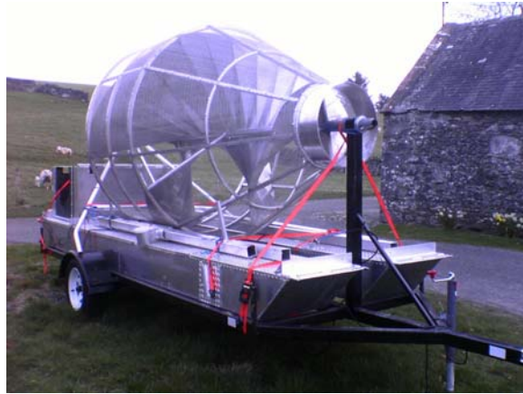
Figure 1: Rotary-screw smolt trap for use on the Bladnoch river (A2Bla10).
